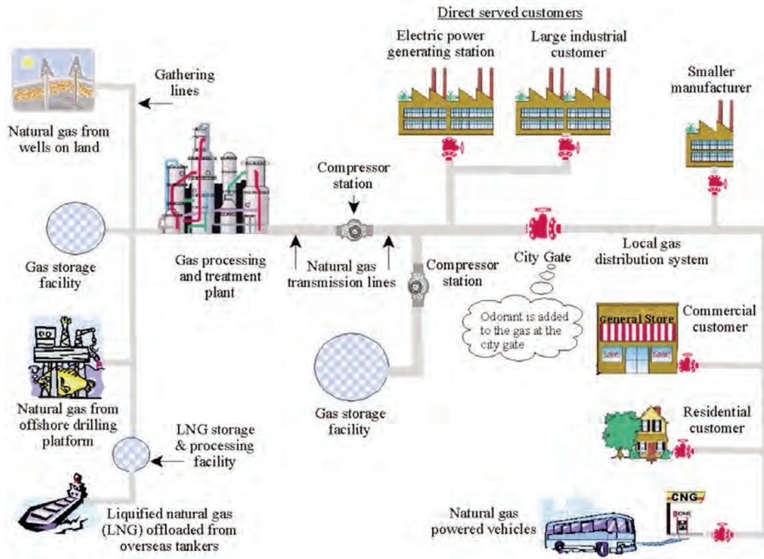
Natural gas pipeline system from production to end user.
